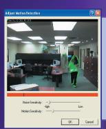
NetDVR incorporates an advanced motion detection algorithm. It alerts the operator to motion that took place while he was not watching the screen. It can draw attention by enhancing motion with bright colors. NetDVR lets you set a schedule to alert you of suspicious motion by cell phone, email and SMS pager.
